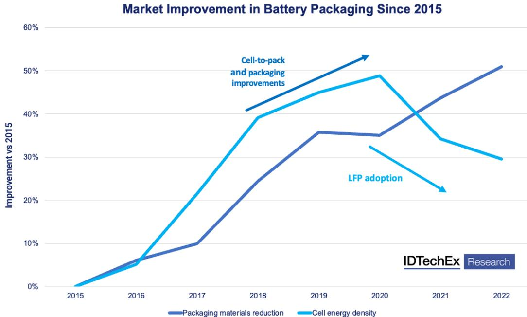
*The increasing share of LFP has decreased average cell energy density, but the efficiency of packaging has continued to increase rapidly, helping offset this at a pack level. Source: IDTechEx*
